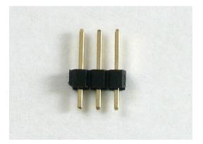
Solder the two small pieces to the **SELO** and **SEL1** pads. These are interface selectors for the chip. Depending on how the jumpers are inserted the chip will talk in TTL serial, i2c or SPI. Also solder a strip to the end so you can plug it into a breadboard.
