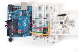
Also, we need to select SPI as the interface so on **SEL1** place the jumper in the **ON** position. for **SEL0** place the jumper in the **OFF** position.
