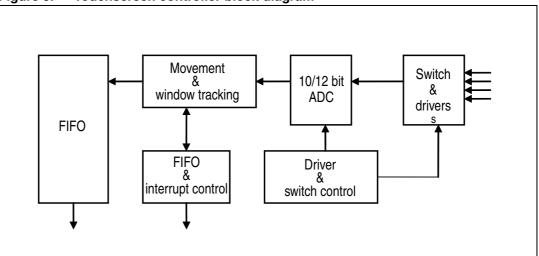
Figure 9. Touchscreen controller block diagram
