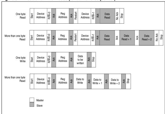
Figure 6. Read and write modes (random and sequential)
