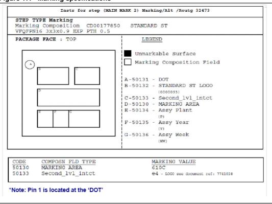
Figure 17. Marking specifications
