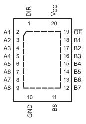
To ensure the high-impedance state during power up or power down,  $\overline{OE}$  should be tied to  $V_{CC}$  through a pullup resistor; the minimum value of the resistor is determined by the current-sinking capability of the driver.
