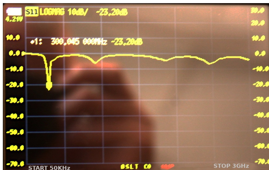
Fig 13: NanoVNA LOGMAX chart of a single pole antenna.
