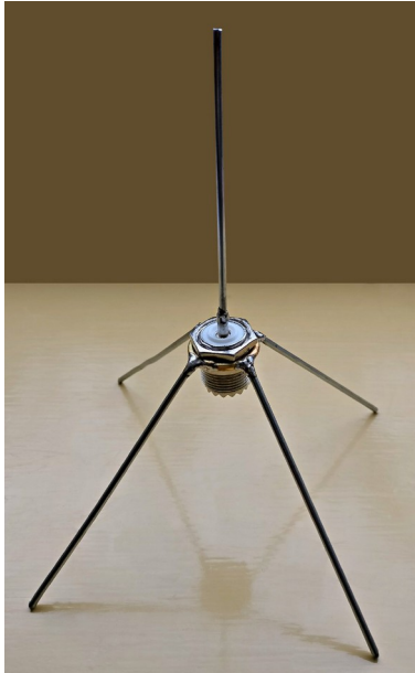
Fig 17: example of single pole antenna with ground plane.
