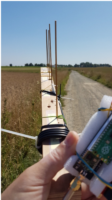
Fig 6: right position of handle on a Yagi antenna
