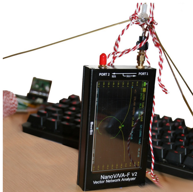
Fig 3: Measuring the power rejected by the antenna to the emitter
