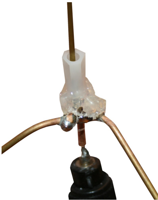
Fig 15: reinforcing the ground plane
