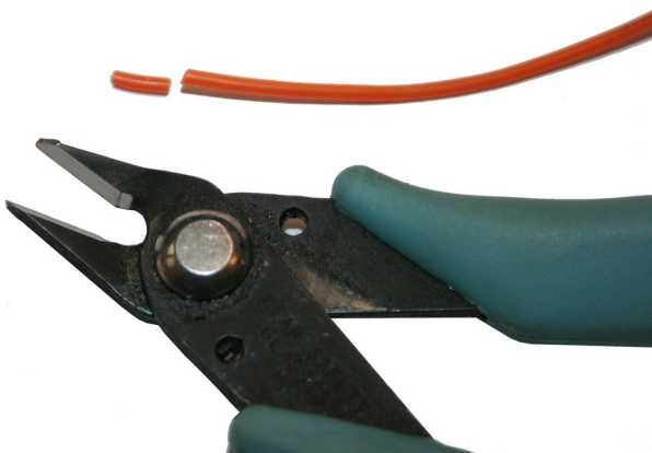
Fig 4: reduce length of antenna
