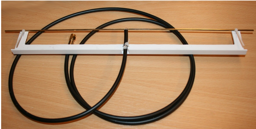
Fig 15: Parasitic mechanical reinforcement
