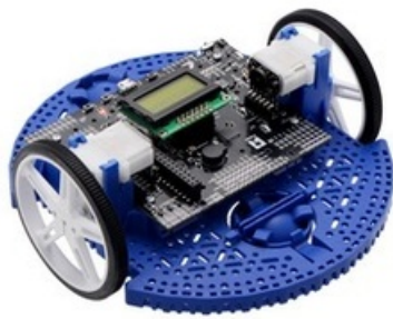
Romi 32U4 Control Board with LCD on a Romi chassis.
